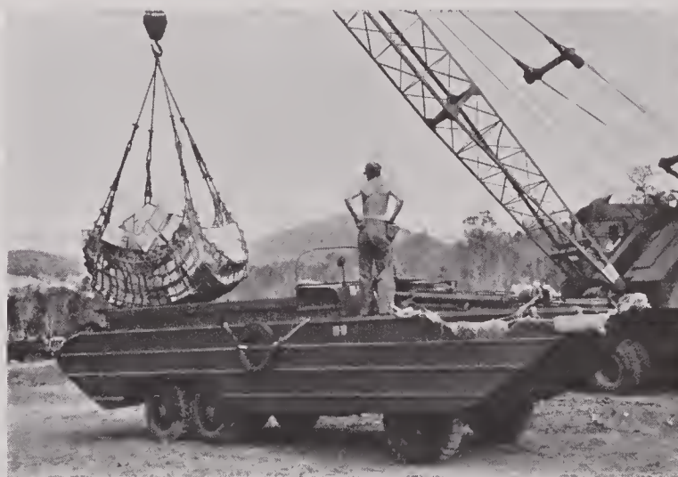
FIGURE 58. Mobile crane lifts cargo from DUKW: simple transfer rig used in Southwest Pacific.
